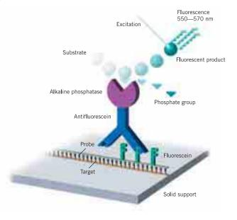
**Fig 33.** Schematic showing the indirect detection of a fluorescein-labelled DNA probe in a Southern blot. The ECF Signal Amplification Module boosts sensitivity by coupling alkaline phosphatase to the fluorescein-labelled DNA probe. Alkaline phosphatase catalyses the formation of stable fluorophores that remain near the probe and emit light when detected using fluorescence imaging systems.
