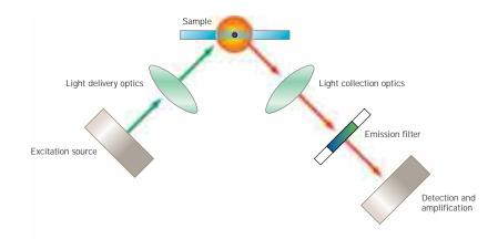
Fig 6. Components of a general fluorescence imaging system.
