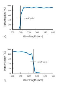
Fig 14. Transmission profiles for a 560 nm long-pass (a) and a 526 nm short-pass (b) filter. The cutoff points are noted.
