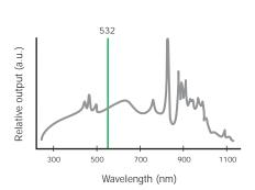
Fig 7. Spectral output of light from a xenon lamp and Nd:YAG laser. The "relative output" axis is scaled arbitrarily for the two light sources. The 532-nm line of the Nd:YAG laser is shown in green.
