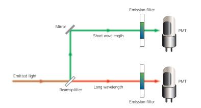
Fig 11. Use of a beamsplitter or dichroic filter with two separate PMTs. Light from a dual color sample enters the emission optics as a combination of wavelengths. A dichroic beamsplitter distinguishes light on the basis of wavelength. Wavelengths above the beamsplitter range pass through, those below are reflected. In this way two channels are created. These two channels can then be filtered and detected independently.
