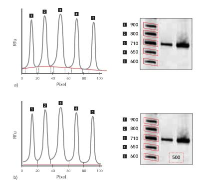
**Fig 29.** Comparison of local and global background correction methods applied to the same image. The local method (panel a) uses different background values at each band in the gel lane, with background based on the average signal from the boundary of each band. In panel b, a single global background value of 500 counts is applied to each band in the analysis.
