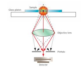
Fig 10. Illustration of confocal optics. Fluorescence from the sample is collected by an objective lens and directed toward a pinhole aperture. The pinhole allows the emitted light from a narrow focal plane (red solid lines) to pass to the detector, while blocking most of the out-of-focus light (black dashed lines).
