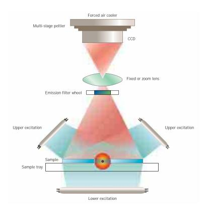
Fig 13. Components of a typical CCD camera-based imaging device. The sample can be illuminated in a variety of ways depending on the nature of the labels to be analysed. The sample is then viewed by the camera. The camera includes focusing optics to accommodate samples at different heights. Emission filters can be inserted in the light path to select specific wavelengths and eliminate background.
