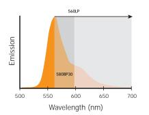
**Fig 17.** Emission filtering of Cy3 fluorescence using either a 580 BP 30 (dark gray area) or a 560 LP filter (light and dark gray areas).
