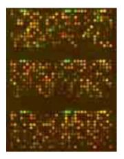
Fig 1. A microarray slide, spotted with DNA from Amersham Biosciences Lucidea<sup>™</sup> Microarray ScoreCard<sup>™</sup> control plate and DNA from Incyte Genomics, Inc. using Amersham Biosciences Generation III Array Spotter, was hybridized with Cy<sup>™</sup>3labelled skeletal muscle cDNA and Cy5labelled liver cDNA. The slide was scanned on Typhoon<sup>™</sup> 9410 Variable Mode Imager with the 10-µm pixel size option.
